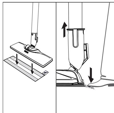
The floor cleaning cloth will stick to the floor nozzle of its own accord due to the hook and loop fastener.
