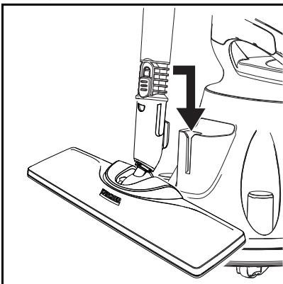
2. Wind the steam hose and mains connection around the carrying handle or device and/or insert the steam gun in the ground floor nozzle.
