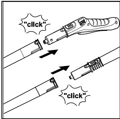
4. Push the accessory and / or the floor nozzle onto the free end of the extension tube.
