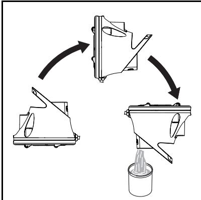
3. Fill a maximum of 1 l distilled water or tap water into the steam boiler.
